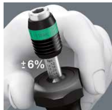
Measurement accuracy is \pm 6\% (article 1430: \pm 10\% ) in accordance with the standard DIN EN ISO 6789. Distinctly audible and noticeable excess-load signal when the pre-set torque is reached.
