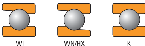
Fig. 21. Angular contact spindle bearing types.
