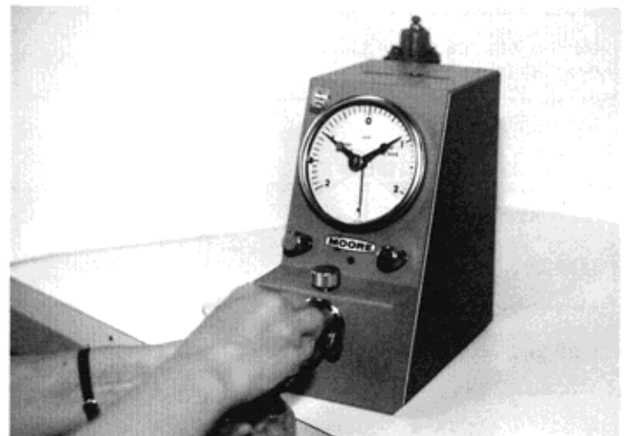
MPB Air Gaging Equipment avoids the distortions of mechanical gaging and assures accurate grading of Bores and OD's.
