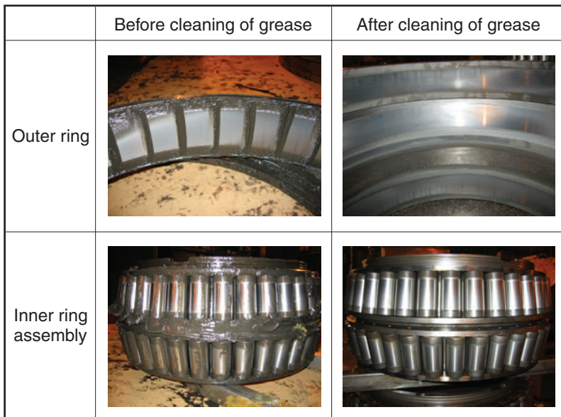
Fig. 5 Post-use appearance of bearing with high-performance seal
