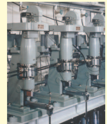
Fig. 1-3 Rolling fatigue life test conditions and test equipment
