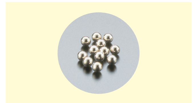
Fig. 2-3 Balls coated with silver ion plating
